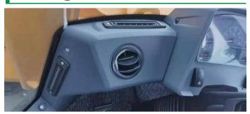
Standard equipped with air conditioning, circulating air enters from the cab, and cold air blows to people's face from the main air outlet in the front, which meets the requirements of human comfort.
