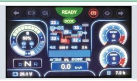
The 7-inch high-definition digital LCD screen displays the motor response, gear position, temperature, pressure, light and etc in real time. Also display all the vehicle falure information and guide the driver to operate.
